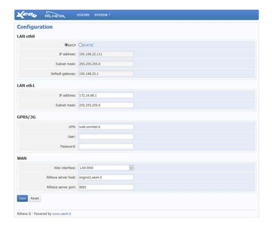
This screen allows to configure the main settings required to perform the startup of the Rilheva device.
